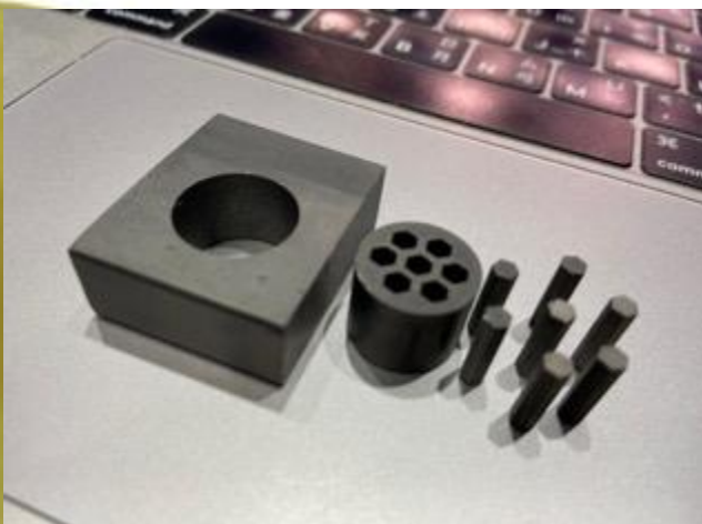
Sintered SiC parts
